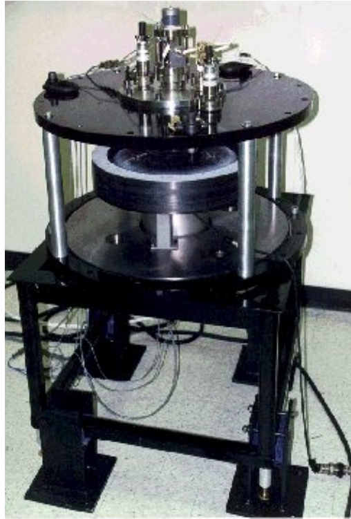
Figure 19 – Example Flywheel Storage System
